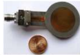
Fig. 4. Fabricated antenna fed by a connector for measurement purpose.
