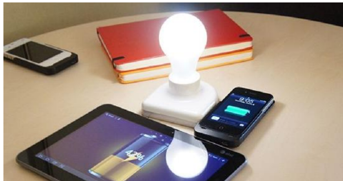
A4WP, Rezenec (Magnetic Inductive coupling)
